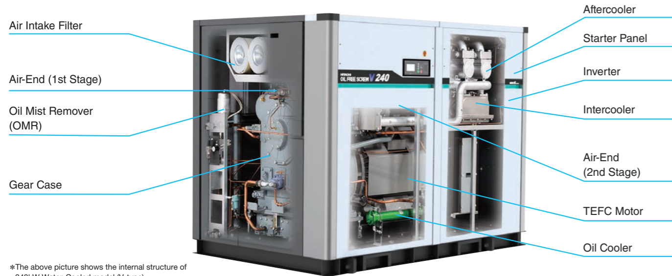
*The above picture shows the internal structure of 240kW Water-Cooled model (V-type).
